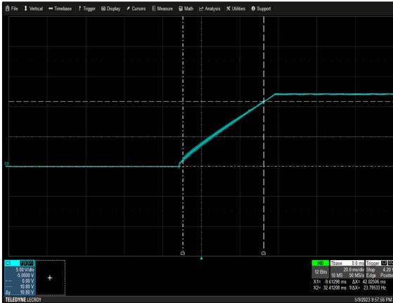
Figure 7: NGB1200S12K Output Voltage Startup Characteristic Vin = 90Vac Load: Io = 100A Ch 3: Vo
