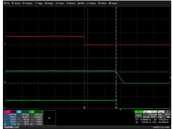
Figure 36: NGB1200S48K Turn Off Characteristic via Control Vin = 115Vac Load: Io = 25A Ch 2: Control Ch 3: Vo Ch 4: POWER_GOOD
