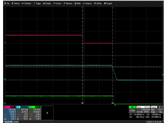
Figure 22: NGB1200S24K Turn Off Characteristic via Control Vin = 115Vac Load: Io = 50A Ch 2: Control Ch 3: Vo Ch 4: POWER_GOOD
