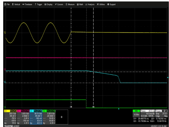
Figure 32: NGB1200S48K Hold-up Time Vin = 115Vac Load: Io = 25A (100% load) Ch 1: V IN Ch 2: V SB Ch 3: V o Ch 4: POWER_GOOD
