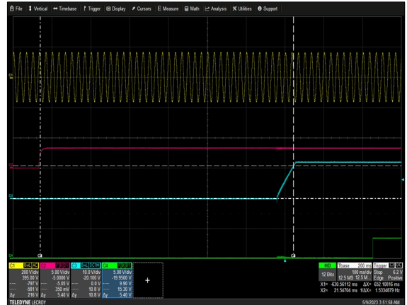
Figure 2: NGB1200S12K Turn-on Delay via Control Vin = 115Vac Load: Io = 100A Ch 1: VIN Ch 2: Control Ch 3: Vo Ch 4: POWER_GOOD
