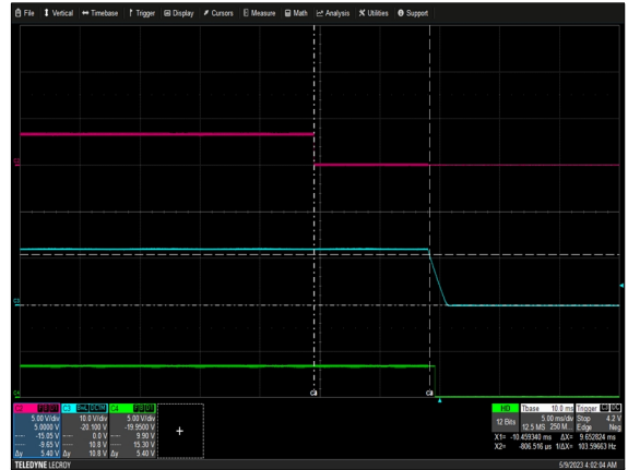
Figure 8: NGB1200S12K Turn Off Characteristic via Control Vin = 115Vac Load: Io = 100A Ch 2: Control Ch 3: Vo Ch 4: POWER_GOOD
