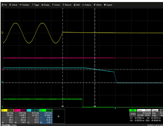
Figure 3: NGB1200S12K Hold-up Time Vin = 115Vac Load: Io = 70A (70% load) Ch 1: VIN Ch 2: VSB Ch 3: Vo Ch 4: POWER_GOOD
