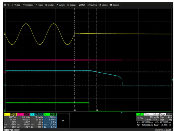
Figure 4: NGB1200S12K Hold-up Time Vin = 115Vac Load: Io = 100A (100% load) Ch 1: VIN Ch 2: VSB Ch 3: Vo Ch 4: POWER_GOOD
