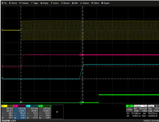
Figure 15: NGB1200S24K Turn-on Delay via AC Mains Vin = 115Vac Load: Io = 50A Ch 1: V IN Ch 2: V SB Ch 3: V O Ch 4: POWER_GOOD
