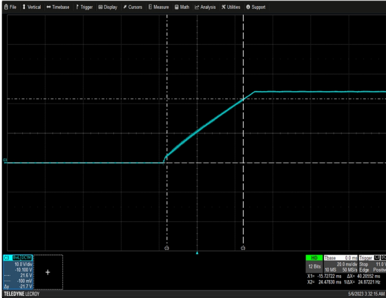
Figure 21: NGB1200S24K Output Voltage Startup Characteristic Vin = 90Vac Load: Io = 50A Ch 3: Vo
