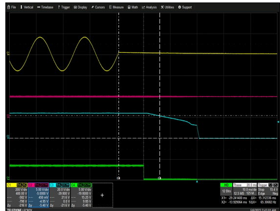
Figure 18: NGB1200S24K Hold-up Time Vin = 115Vac Load: Io = 50A (100% load) Ch 1: V IN Ch 2: V SB Ch 3: V O Ch 4: POWER_GOOD
